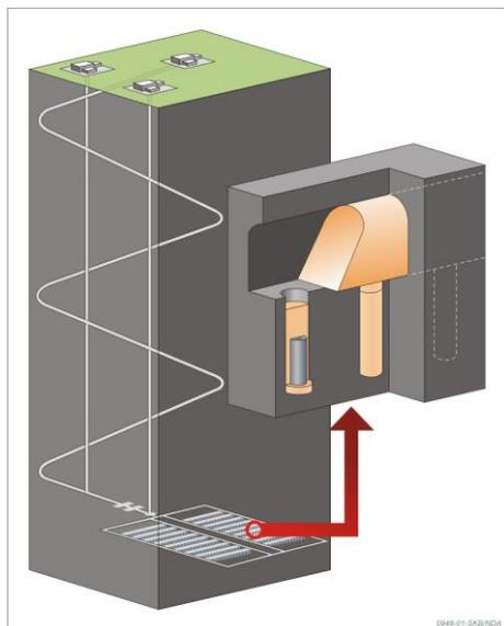
Figure 1 Generic disposal concept for HHGW in higher strength crystalline rock
