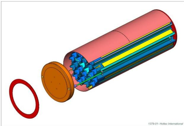
Figure 3 Generic Multi-Purpose Container for storage, transport and disposal of spent fuel
