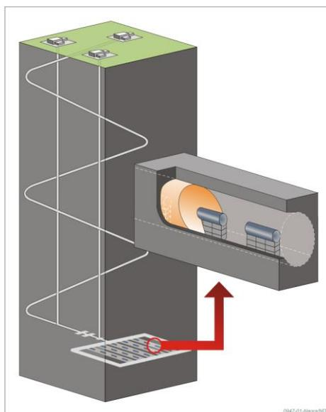
Figure 2 Generic disposal concept for HHGW in lower strength sedimentary rock
