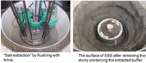
Fig. 14 A full scale demonstration experiment of retrievability technology for a pit disposal concept<sup>14</sup>
