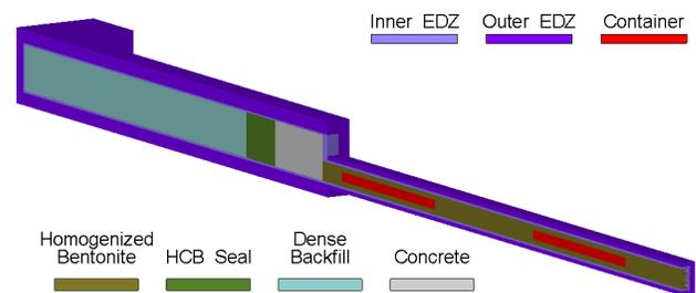
Fig. 1. Detail of Room-Scale Model showing sealing materials and EDZ in room entry and first 10 containers (2 container elements).
