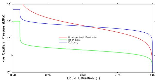
Fig. 3. Capillary Pressure Curves for Placement Room Bentonite (Homogenized Bentonite), Repository Inner EDZ, and the Cobourg Formation
