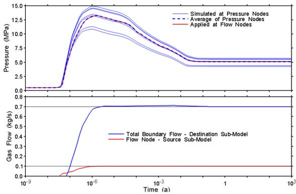
Fig. 11. Verification model pressure and flow results
