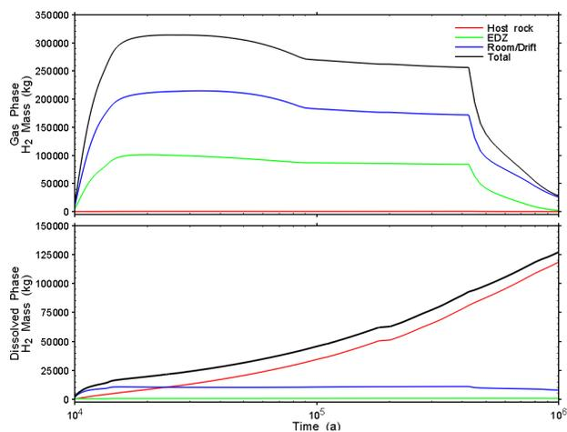
Fig. 5. Room-Scale Model gas allocation (scaled for full repository)
