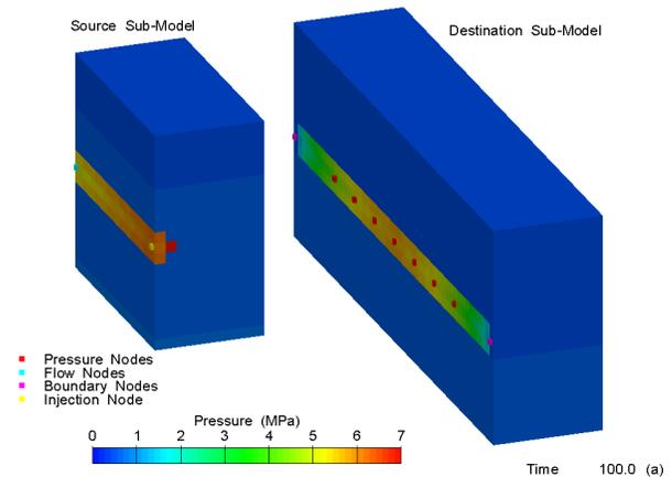
Fig. 10. Pressure distribution at 100 a
