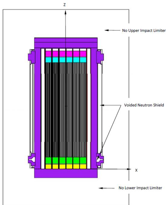
**Figure 6 - X-Z VISED Plot of ENUN 32P HAC MCNP5 Model**
