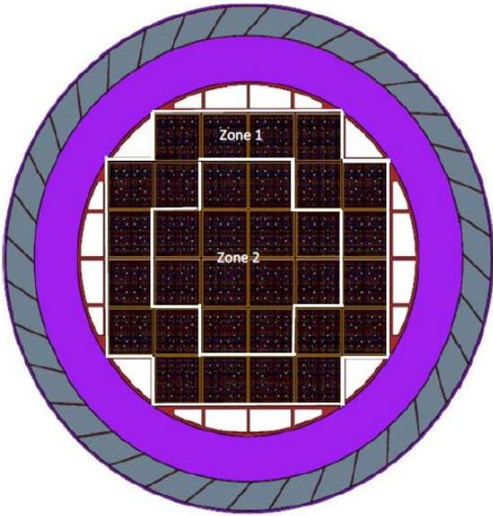
Figure 1 – ENUN 32P Zonal Loading Arrangement
