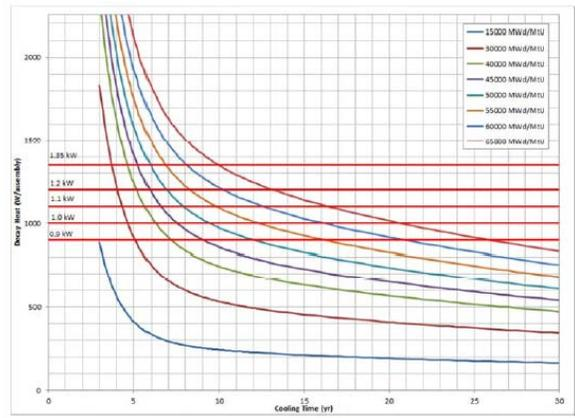
Figure 2 - Design Basis KWU 16x16 Fuel Assembly Decay Heat Characteristics
