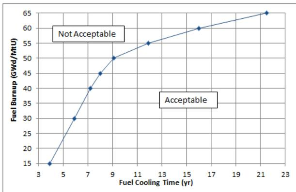
**Figure 10 - ENUN 32P Burnup and Cooling Time Loading Curve for Zonal Loading - Zone 1 - Westinghouse 17x17**
