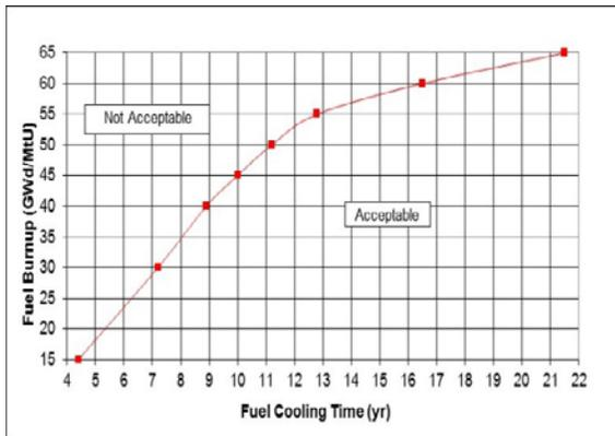
**Figure 9 - ENUN 32P Burnup and Cooling Time Loading Curve for Zonal Loading - Zone 1 - KWU**
