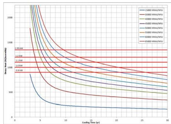
Figure 3 - Design Basis Westinghouse 17x17 Fuel Assembly Decay Heat Characteristics
