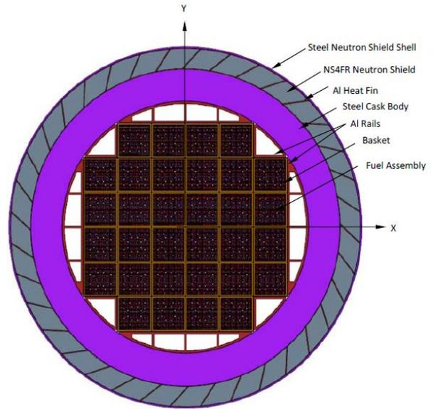
Figure 4 - X-Y VISED Plot of ENUN 32P NCT MCNP5 Model
