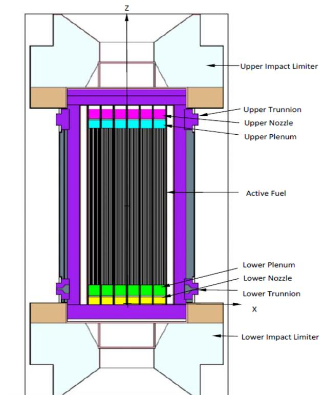
Figure 5 - X-Z VISED Plot of ENUN 32P NCT MCNP5 Model
