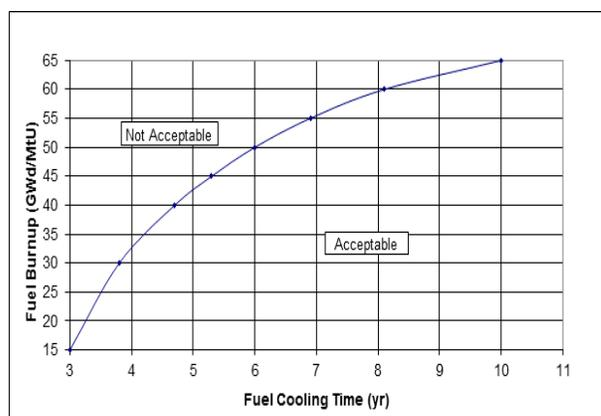
**Figure 7 - ENUN 32P Burnup and Cooling Time Loading Curve for Zonal Loading - Zone 2 - KWU**
