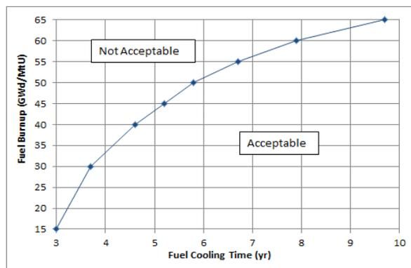
**Figure 8 - ENUN 32P Burnup and Cooling Time Loading Curve for Zonal Loading - Zone 2 - Westinghouse 17x17**
