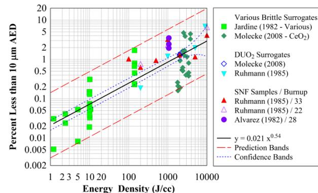
Fig. 3. Mass of aerosols with aerodynamic equivalent diameter (AED)  $< 10 \mu\text{m}$  normalized by affected mass as a function of energy density.
