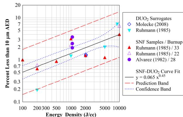
Fig. 4. Mass of SNF and  $\text{DUO}_2$  aerosols with aerodynamic equivalent diameter (AED)  $< 10 \mu\text{m}$  normalized by affected mass as a function of energy density.
