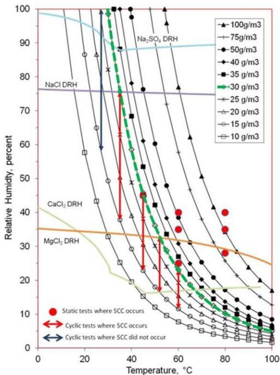
Figure 2. Relative humidity vs. temperature diagram for varying absolute humidity values. Deliquescence behavior of sea salt components and U-bend CISCC tests reported in NUREG/CR-7170 are shown as a function of temperature [3].
