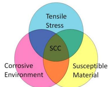
Figure 1. Venn Diagram showing the necessary components for stress corrosion cracking.
