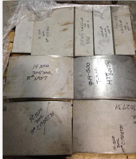
Fig. 1. Stainless steel materials used to fabricate dry storage canister flaw mockups for demonstration and qualification purposes.
