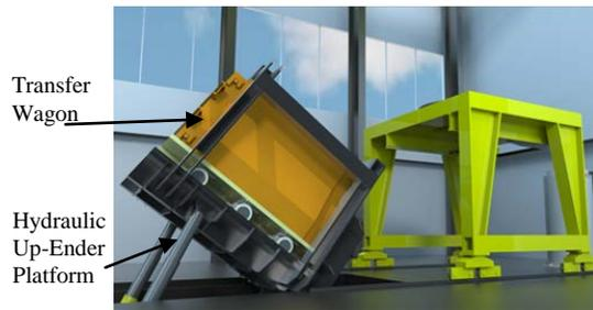
Fig. 6. Vertical to vertical transfer station.
