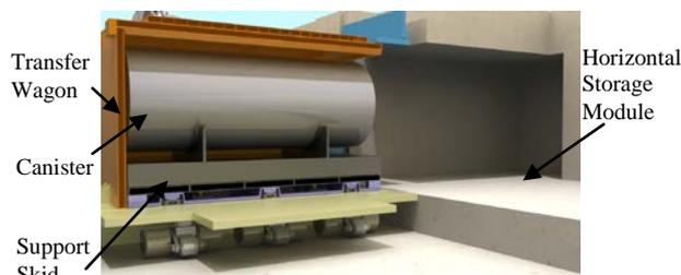
Fig. 9. Loading canister to horizontal storage module.
