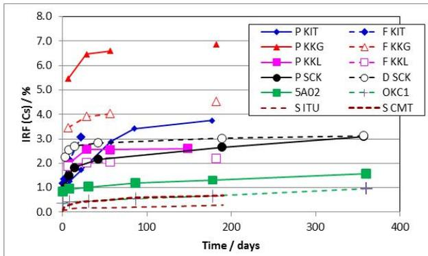
Fig. 3. Measured cumulative <sup>137</sup>Cs release from various SNF samples:
