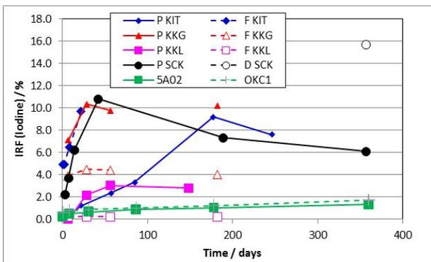
Fig. 4. Measured cumulative <sup>129</sup>I release from various SNF samples. (Nomenclature see Fig. 3). Uncertainty of <sup>129</sup>I measurements: ±20 %.
