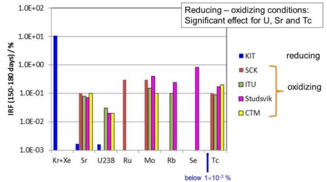
Fig. 5. Cumulative elemental releases from various SNF samples under oxidizing, anaerobic and reducing conditions. (KIT: reducing conditions).
