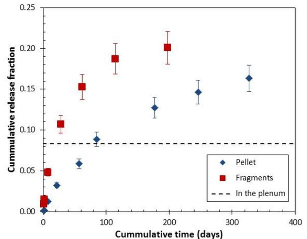
Fig. 2. Cumulative release fraction of FG (Xe+Kr) as function of time during leaching of SNF (50.4 GWd/t<sub>HM</sub>) in comparison to the FGR into the plenum of the rod[11].
