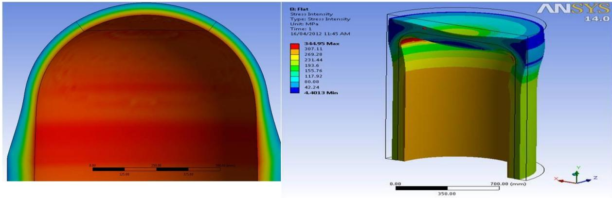
**Figure 2 Stresses in a spherical vs. a flat head**
