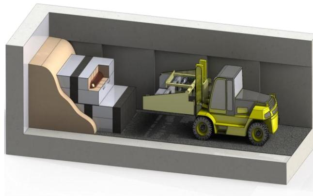
**Figure 8 Canadian slip skid emplacement system**
