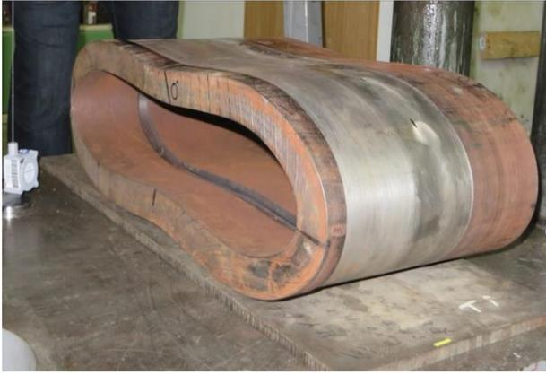
**Figure 4 Weld ring crush test**
