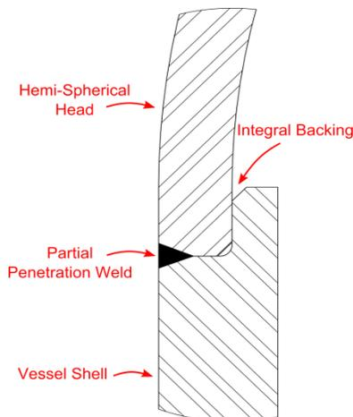
**Figure 3 Partial penetration weld design**
