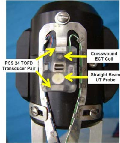
Fig. 5. Photograph of low-profile “blade” probe for examination of CRDM penetration tubes behind thermal sleeves.<sup>16</sup>
