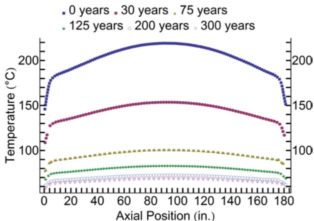
Fig. 3. Temperature profiles along the length of a horizontal canister from loading to 300 years of storage assuming 32 PWR fuel assemblies and initial heat load of 41 kW.<sup>1</sup>
