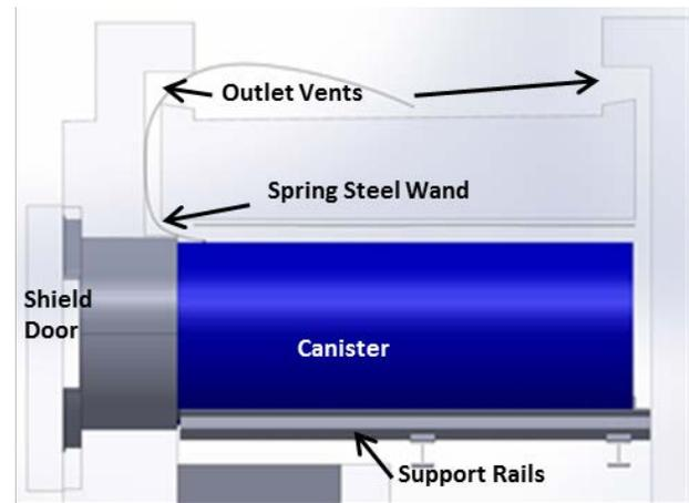
Fig. 2. Illustration of NDE accessibility to canister surface through outlet vent in horizontal dry storage system.<sup>1</sup>
