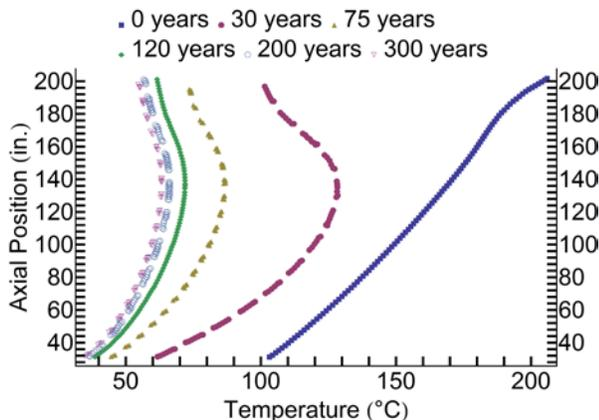
Fig. 4. Temperatures profiles along the length of a vertical canister from loading to 300 years of storage assuming 32 PWR fuel assemblies and initial heat load of 30 kW.<sup>1</sup>
