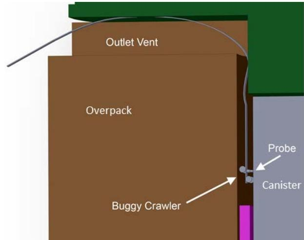
Fig. 1. Illustration of NDE accessibility to canister surface through outlet vent in vertical dry storage system.<sup>1</sup>
