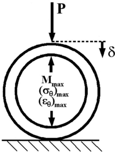
Fig. 1. RCT loading ( $P$ ) and controlled displacement ( $\delta$ ).
