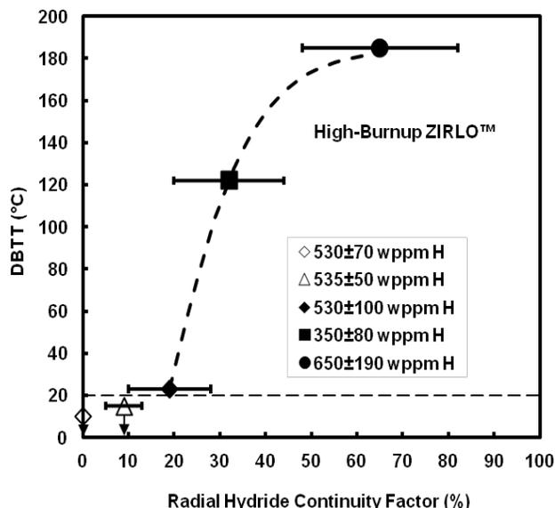
Fig. 3. DBTT as a function of RHCf for HBU ZIRLO™.
