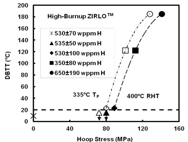
Fig. 2. DBTT as a function of 400°C RHT hoop stress (solid symbols) and hoop stress at 335°C (open symbols).
