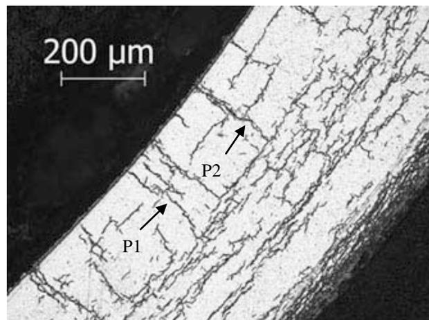
Fig. 4. 100X image of HBU ZIRLO™ sample 648C7 at the 4:30 o'clock orientation.
