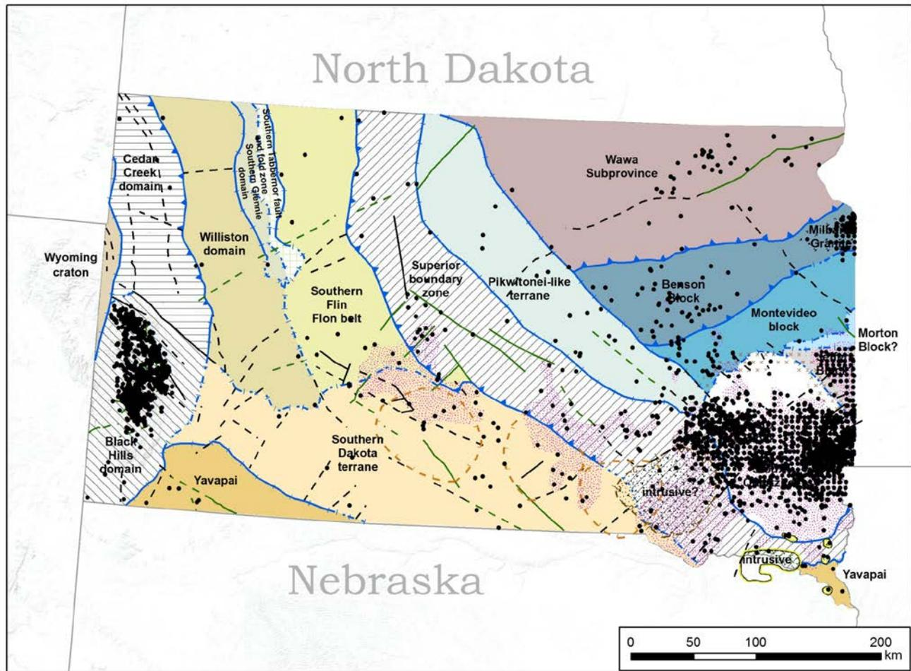
Fig. 4. Basement terrane and structure map of South Dakota.<sup>10</sup> Solid black circles represent the location of boreholes that penetrated Precambrian basement rocks. Granite was the most common lithology encountered within the crystalline basement.
