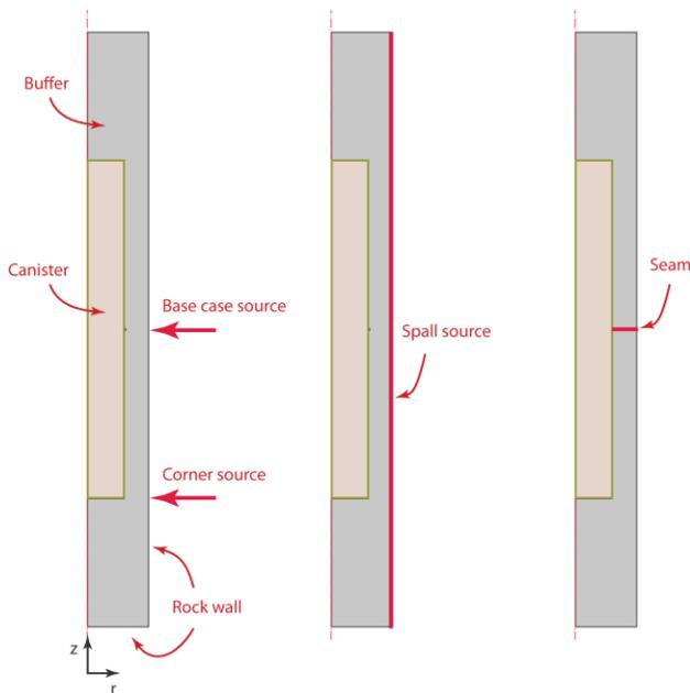
Fig. 1. Schematic description of 2D radial model geometry for the deposition hole and canister, including source location scenarios.
