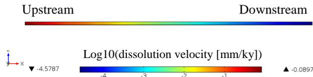
Fig. 4. Rate of copper removal along the 9.2-cm strip of a 1-mm diameter pipe where it grazes the canister. The color scale indicates instantaneous dissolution velocity; extremes values are indicated with triangles. Flow is from left to right.
