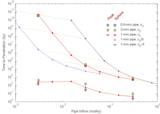
Fig. 5. Time to penetrate 5 cm of copper given pipe supply of sulphide at (i) the initial peak dissolution rate and (ii) with diffusion-limited growth of a hemispherical shell.
