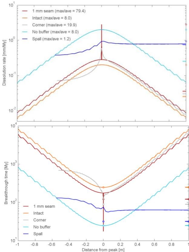
Fig. 2. Spatial distribution, relative to the peak location, of (top) instantaneous corrosion rate and (bottom) corresponding time to penetrate a 5-cm copper thickness given a  $10^{-5}$  mol/L sulphide background concentration. Symbols on right axis of (top) indicate peaks (circles) and averages across the entire canister surface (bars). Circles in (bottom) indicate average corrosion rate, correcting for radial diffusion at corners and seam endpoint.
