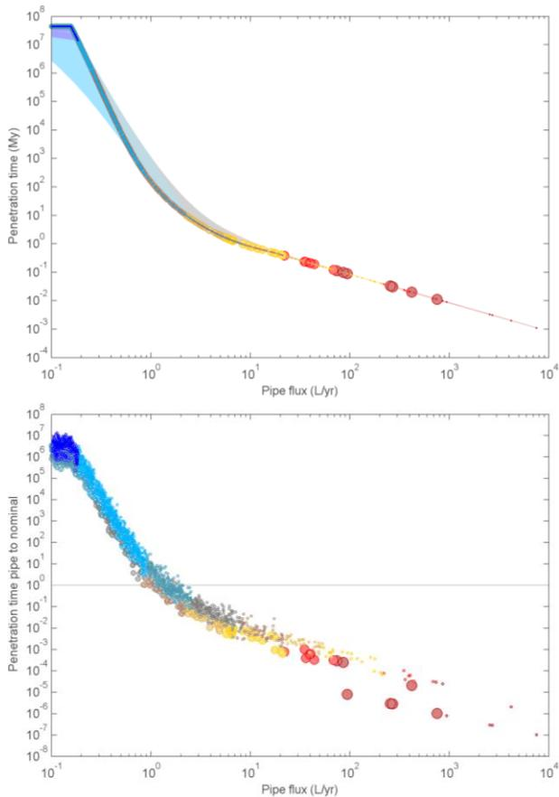
Fig. 8. (top) Estimated penetration time as a function of volumetric flux in the pipe for spherical dissolution at the pipe/copper contact. (bottom) Ratio of penetration times for pipe flow relative to the nominal intact buffer scenario with a 1-mm fracture (see Fig. 2).
