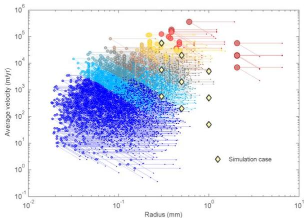
Fig. 7. Scatter plot of limiting pipe radius and velocity given fracture fluxes and gradients at deposition holes. Symbols use the color scheme from Fig. 6. Lines illustrate the consequence of reducing pipe gradient one order of magnitude relative to background with flux capture multiplied by 1 (slant) and 10 (horizontal).
