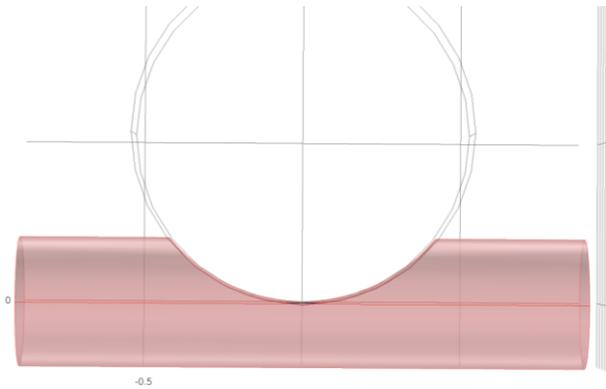
Fig. 3. Geometry of the pipe simulation. The highlighted zone is the simulation domain, representing a bentonite cylinder cut by a canister. The pipe is located at the bentonite cylinder centerline. Deposition-hole boundaries are neglected at the ends of the simulation domain.
