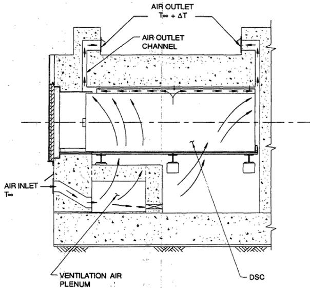
Figure 1. NUHOMS<sup>®</sup> Dry Cask Storage System Showing Air Flow<sup>6</sup>
