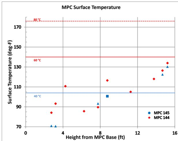
Figure 4. Hope Creek Canister Side Measured Temperatures
