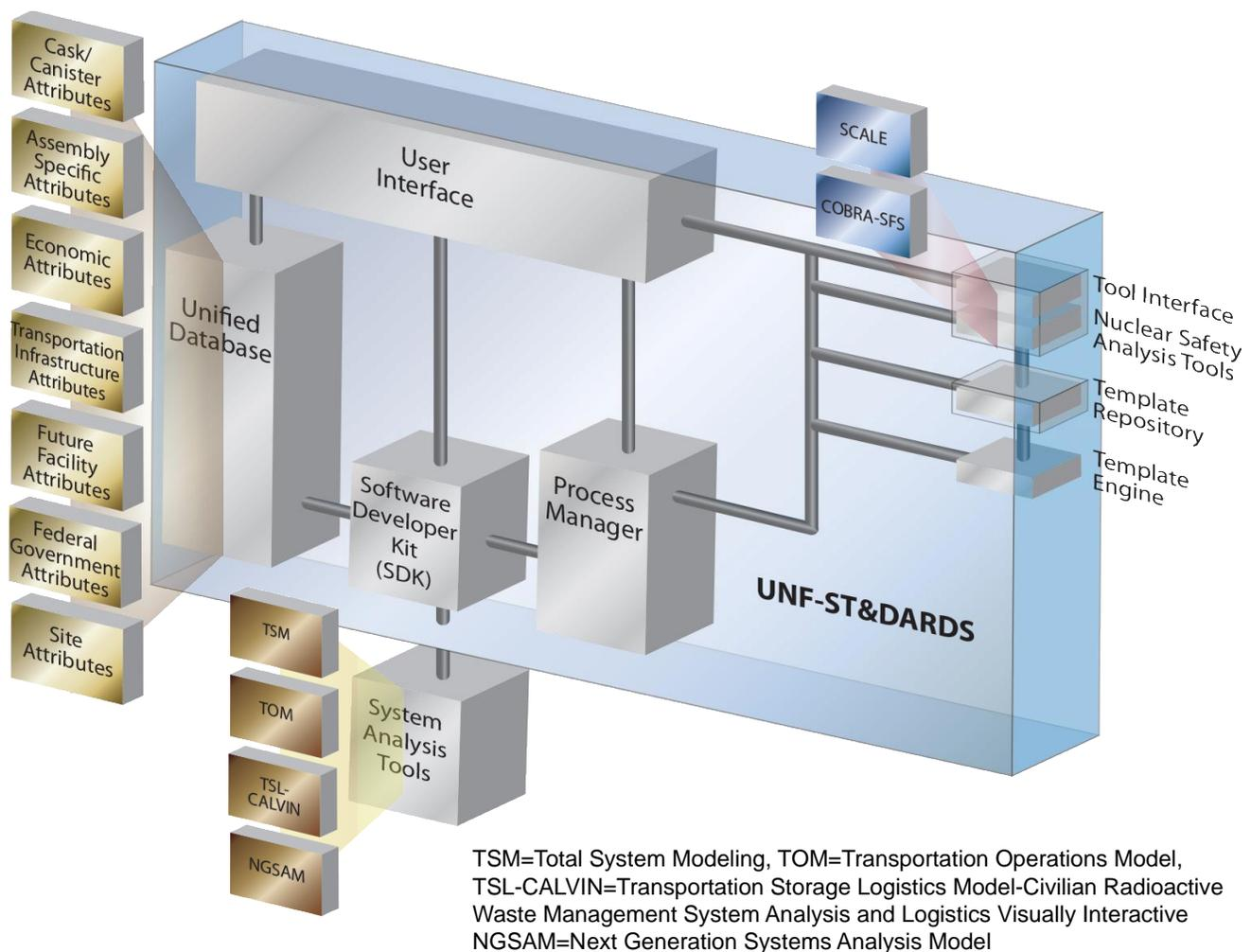
Fig. 1. Components of the UNF-ST&DARDS.
