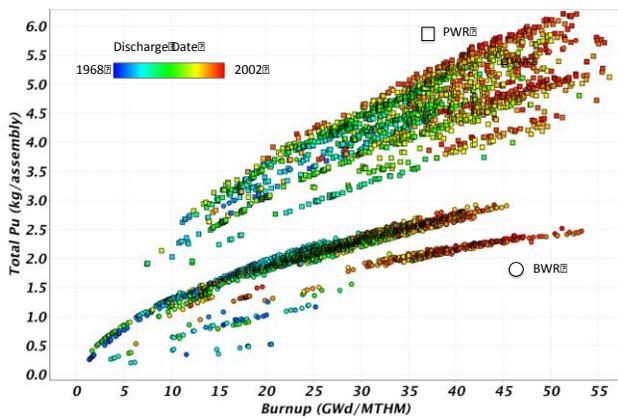
Fig.4. Quantity of plutonium per assembly from a discharged SNF assembly as a function of burnup per assembly and reactor type evaluated at 2025.
