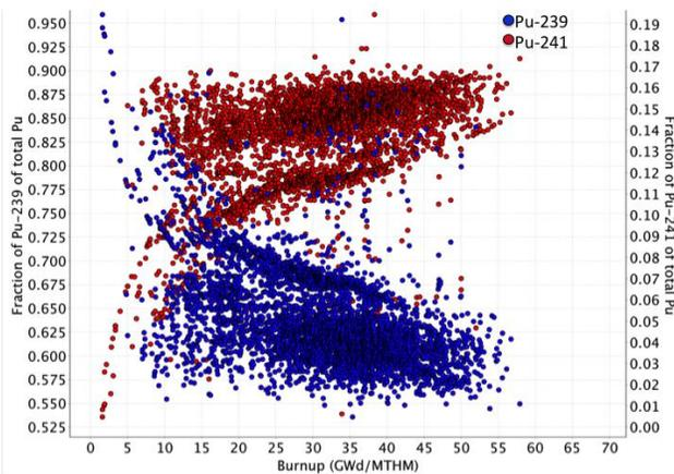
Fig. 5. Percentage of Pu-239 and Pu-241 within a SNF assembly at assembly discharge as a function of burnup.
