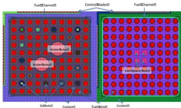
Fig. 2. GE4610G14 assembly type (left), XCL10a assembly type (right).
