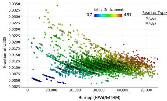
Fig. 3. Enrichment of uranium from a discharged SNF assembly as a function of burnup and reactor type.
