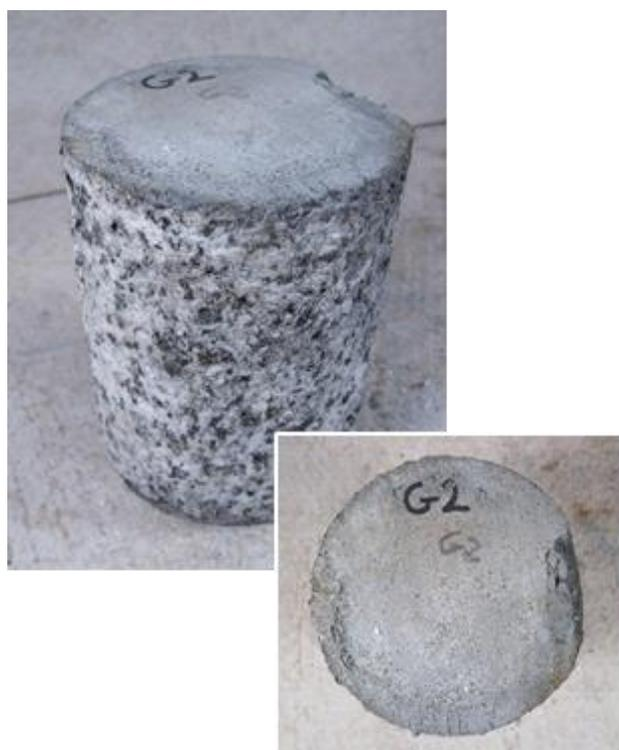
Figure 2. Thermal plug sample removed from granite block test (7.6 cm diameter plug, high dilution of thermite with aluminum oxide)
