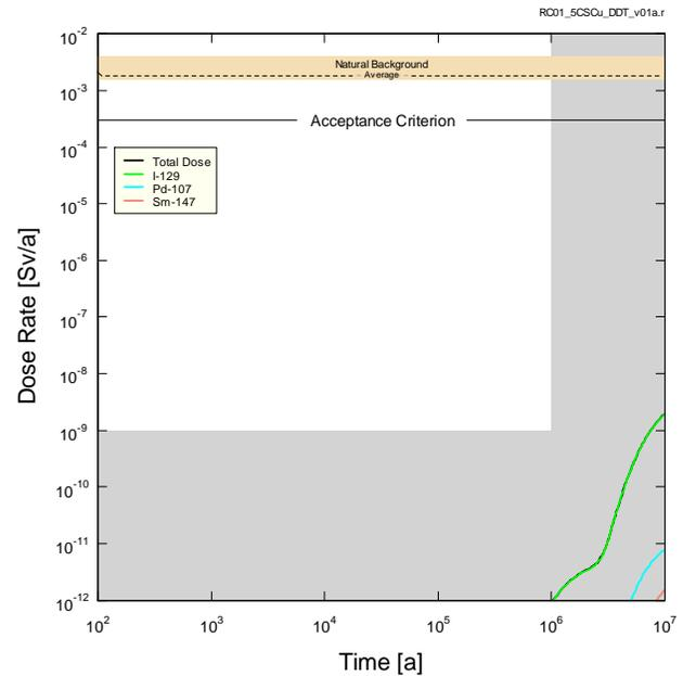
Fig. 8. SYVAC3-CC4 – Reference Case Individual Radionuclide Dose Rates
