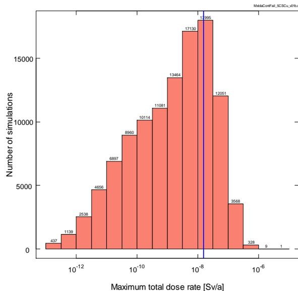
Fig. 11. Distribution of the Maximum Dose Rate for Simulations with at Least One Defective Container
