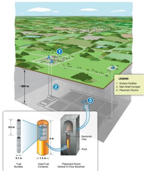
**Fig. 1. Crystalline Rock Repository Design**
