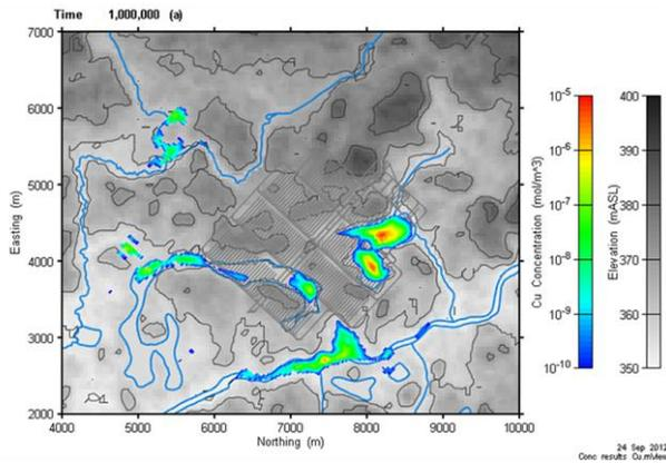
**Fig. 9. FRAC3DVS-OPG – Copper Concentration over the Repository Site**
