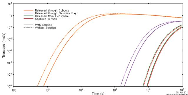
**Fig. 10. FRAC3DVS-OPG – Copper Transport to the Surface both with and Without Sorption**
