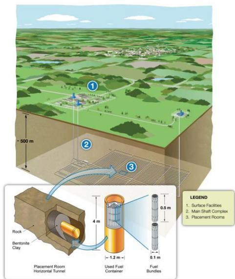
**Fig. 2. Sedimentary Rock Repository Design**
