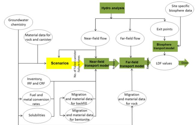
Fig. 1 Models and data for the consequence calculations (Modified based on SKB, Ref. 1).
