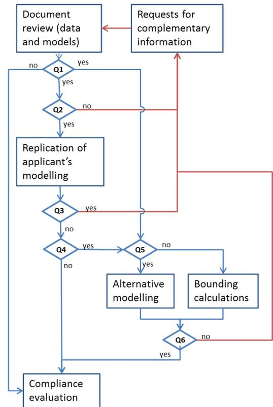
Fig. 6 Schematic of the integrated modelling approach for regulatory review of a consequence analysis, with the following decision points: Q1: Necessary to reproduce? Q2: Feasible to reproduce? Q3: Any errors or ambiguities identified? Q4: Any remaining unresolved review issues, e.g. conceptual model uncertainty? Q5: Does SSM have access to an alternative model? Q6: Sufficient understanding for compliance evaluation? See text for details.
