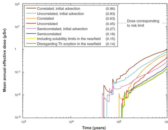
Fig. 5 Summary of far-field mean annual effective dose for uncertainty calculations performed for the corrosion scenario. The peak doses are given in parentheses in  $\mu\text{Sv}$  (From SKB, figure 13-40 in Ref. 1)
