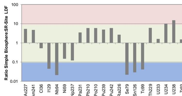
Fig. 7 Maximum dose factors for groundwater release to combined agricultural land with a deep well compared with SR-Site basic LDFs (Ref. 26). Results for 20 out of 39 radionuclides are displayed.
