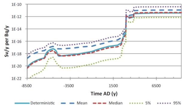
Fig. 3 Evolution of the LDF in time for Ra-226, showing the effect of uncertain parameters. The deterministic LDF values are also shown for comparison. (From SKB, figure 5-36 in Ref. 9).
