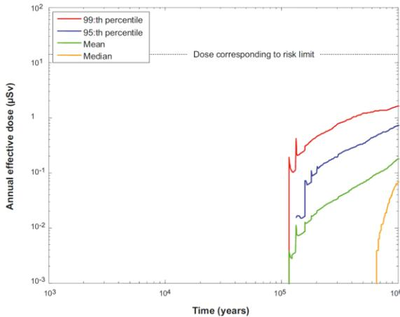
Fig. 4 Far-field annual effective doses (mean, median, 95<sup>th</sup> and 99<sup>th</sup> percentiles) for the probabilistic calculation of the central corrosion case (From SKB, figure 13-19 in Ref. 1).
