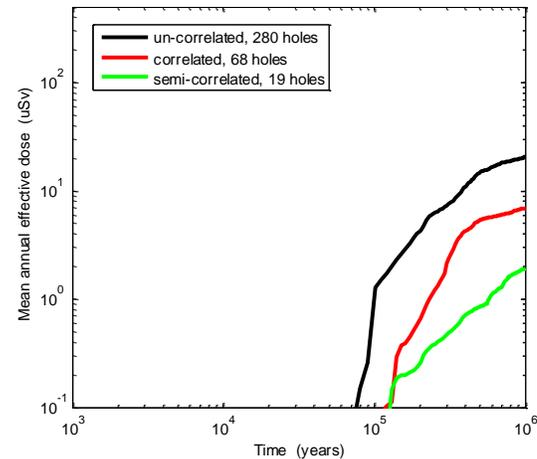
Fig. 8 Far-field annual effective dose for bounding cases calculated probabilistically for corrosion cases.
