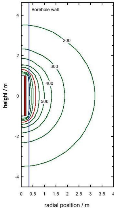
Fig. 5. Isotherms of peak temperatures generated in the scenario illustrated in Fig. 4. The 700°C (red) isotherm corresponds to the solidus temperature for the granite shown in Fig. 1<sup>10</sup>.
