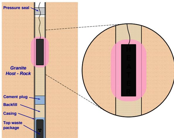
Fig. 3. Schematic of the rock welding concept for sealing a deep borehole disposal (not to scale).
