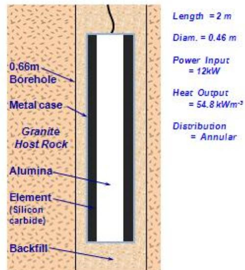
Fig. 4. Schematic of a possible rock welding scenario for a 0.66 m diameter borehole using a hollow cylindrical heater.
