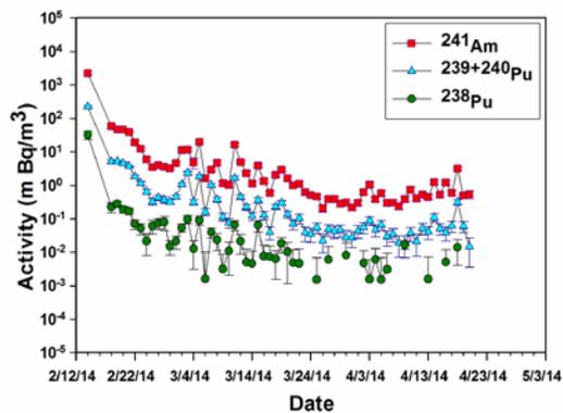
Fig. 3. The daily  $^{241}\text{Am}$ ,  $^{239+240}\text{Pu}$  and  $^{238}\text{Pu}$  concentrations in Station A (Pre-HEPA, Top) and Station B (Post-HEPA, Bottom) filters following the February 14, radiation release event at the WIPP.
