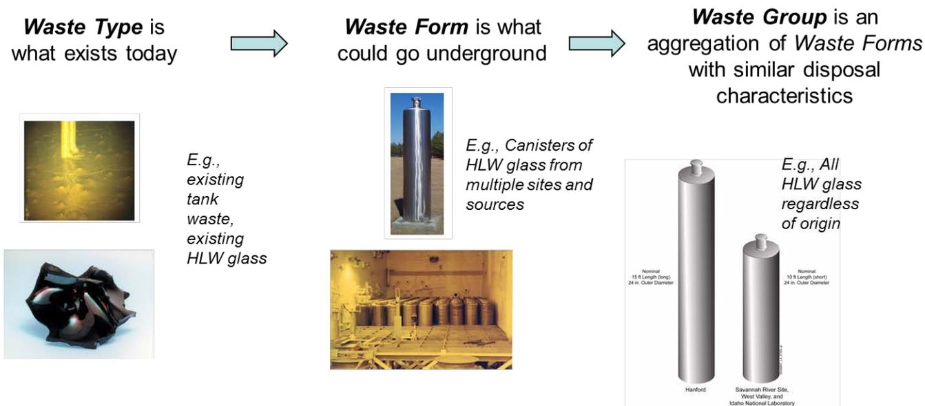
Figure 2. Examples of “waste type,” “waste form,” and “waste group” using high-level radioactive waste glass.
