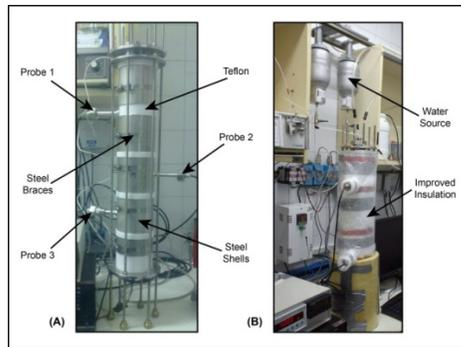
Fig. 1. Column test cell (A) before being wrapped with the insulation material and (B) with improved insulation.
