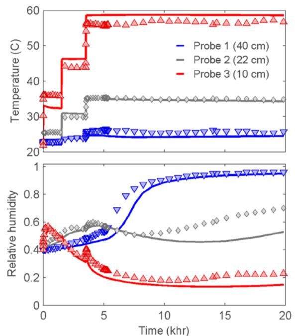
Fig. 5. Time history of temperature and RH at probe locations over the thermal and injection phases. Symbols indicate laboratory measurement and lines indicate model results.
