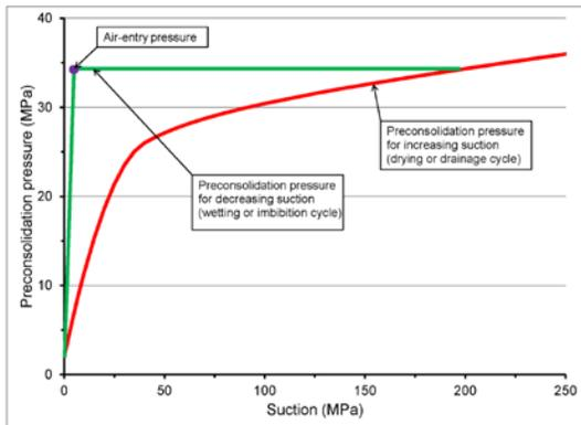
Fig. 2. Preconsolidation pressure  $P_c$  versus suction  $s$  model based on  $P_{co} = 2$  MPa [For saturated condition, based on data from Rizzi, et al.<sup>10</sup>] and suction pressure.
