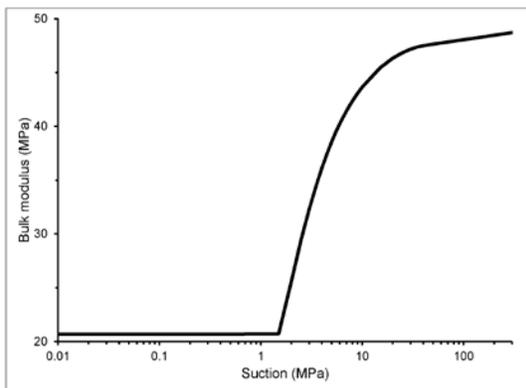
Fig 3. Bulk modulus  $K$  versus suction  $s$  model (based on  $K-p$  relationship<sup>14</sup> and parameter values described in this paper).
