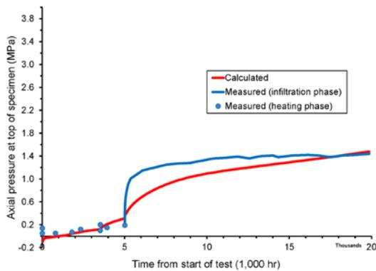
Fig. 7. Calculated and measured axial pressure histories at the top of the bentonite column over the thermal and injection phases.
