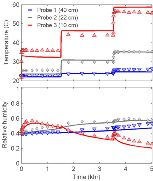
Fig. 4. Time history of temperature and RH at probe locations over the thermal phase. Symbols indicate laboratory measurements and lines indicate model results.
