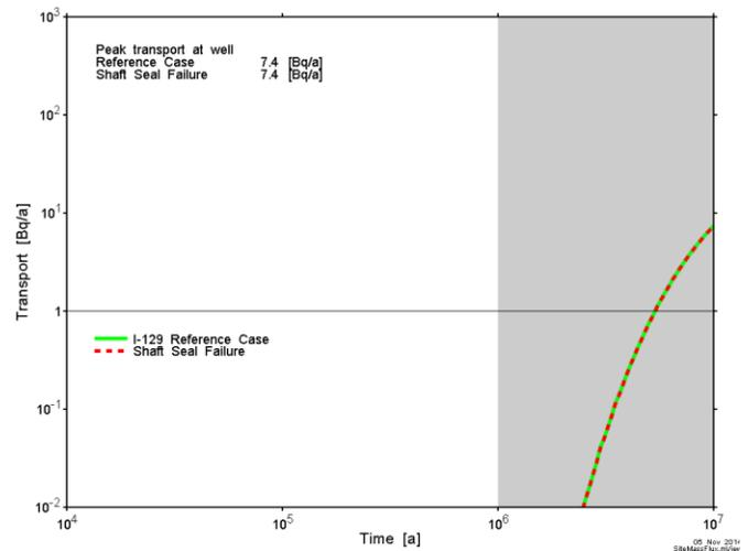
Fig. 6. I-129 Transport to the Well for Shaft Seal Failure Scenario.
