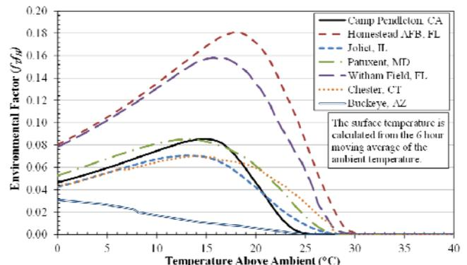
Fig. 2. Average of the Environmental Factor on CGR ( $f_T f_H$ ) Based on One Year of Hourly Climate Data
