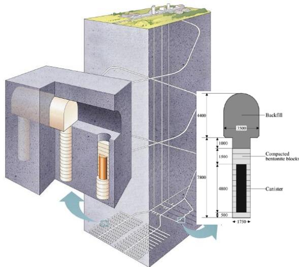
Fig. 1. Schematic of KBS-3 vertical emplacement concept (compiled from Refs. 3-8).
