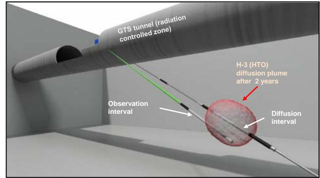
Figure 8: Schematic illustration of the LTD Phase 2 *in situ* test consisting of surface equipment in the GTS radiation controlled zone, injection borehole (17 m) and observation borehole (15 m).
