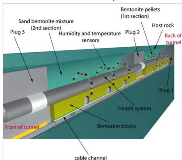
Figure 10: The HE-E experiment layout
