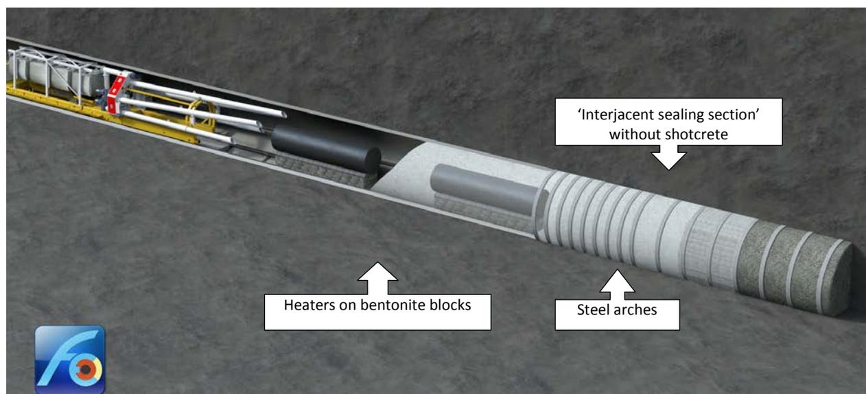
Figure 11: Visualization of the general experimental layout of and backfilling procedure of FE (diameter 3 m), as well as, the developed prototype machine with five auger conveyors used for the backfilling. The longest auger is 8.5m long.
