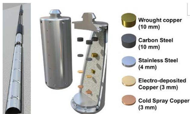
Figure 4: Experimental layout: Borehole with modules; cutaway of one module showing the distribution of metal coupons.
