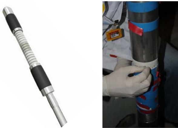
Figure 7: Schematic of CFM Long-term In-situ test packer system (left), showing in grey the four traced pre-compacted bentonite rings with 10% synthetic montmorillonite (Zn labelled) and photograph (right) of the emplacement of the tracer vials (length of test interval with bentonite rings: 40 cm long).
