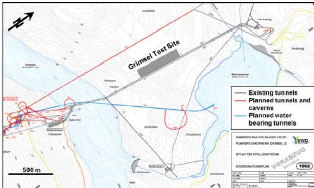
Figure 5: Map of Grimsel area with outline of the existing and planned excavations (courtesy of KWO). Lake Raeterichsboden is the lake to the right on the figure.
