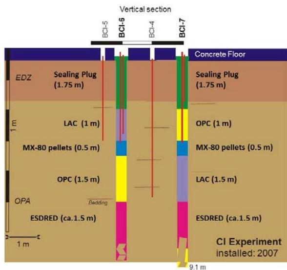
Figure 12: Overview of the Cement-Clay interaction experiment showing two boreholes filled with segments of Bentonite, Low Alkali Cement (LAC), Ordinary Portland Cement (OPC) and ESDRED Low-pH cement.
