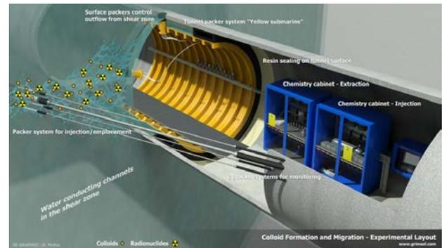
Figure 6: Schematic illustration of the layout of the long-term in-situ test initiated in the framework of CFM in May 2014 (gallery diameter 3.5 m)
