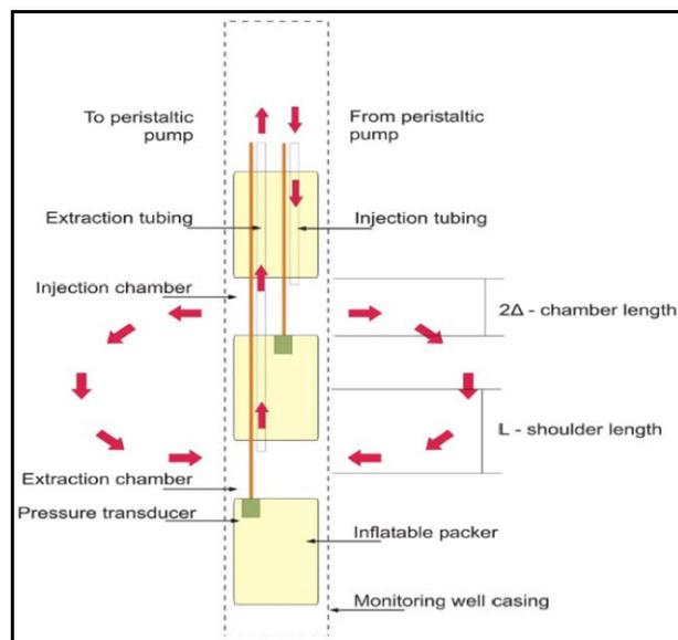
Fig. 2. Schematic Diagram of the Vertical Dipole Tracer Test Configuration<sup>13</sup>.
