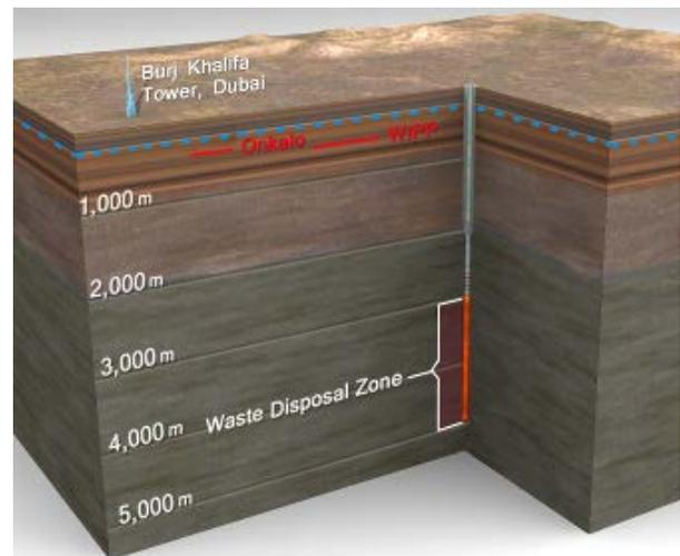
Fig. 1. Generalized concept for Deep Borehole Disposal of radioactive waste<sup>5,6</sup>; dashed blue line indicates lower limit of typical fresh water
