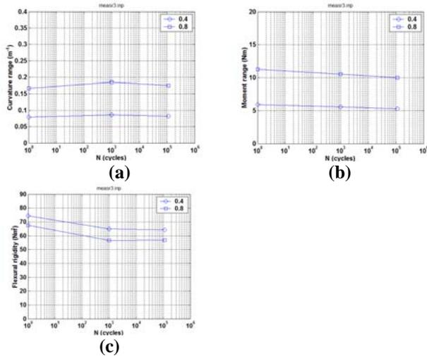
Fig. 3. Variations of (a) curvature range, (b) applied moment range, and (c) flexural rigidity as a function of number of cycles for D13/R3 (606B3E);  $N_f = 1.29 \times 10^5$  cycles under  $\pm 13.72 \text{ N}\cdot\text{m}$  5 Hz.
