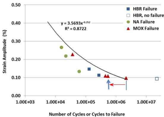
Fig. 15. Strain amplitudes as a function of number of cycles; results are based on CIRFT testing at 5 Hz. The power function was obtained from curve fitting based on the HBR data set [5]. The data point with the arrow represents two-foot drop test applied to CIRFT specimen before the dynamic vibration test being carried out.
