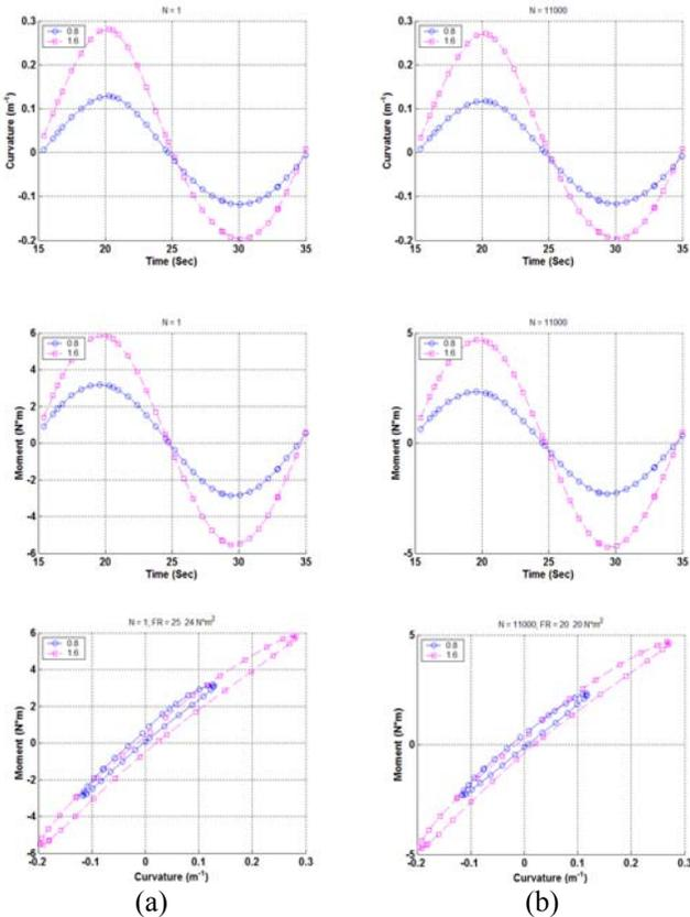
Fig.11. Moment and curvature as a function of time and moment-curvature loops based on measurements when (a)  $N=1$  and (b)  $N=111,000$  cycles for MOX2 (MOX-A-12). Measurements were made with 0.8 and 1.6 mm relative displacements;  $N_f = 3.7 \times 10^4$  cycles under  $\pm 10.16 \text{ N}\cdot\text{m}$ , 5 Hz.
