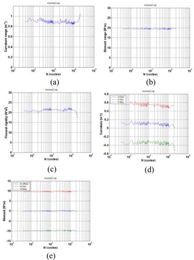
Fig. 9. Variations of (a) curvature range, (b) applied moment range, (c) flexural rigidity, (d) maximum and minimum values of curvature, and (e) maximum and minimum values of moment as a function of number of cycles for NA2 (651C5);  $N_f = 2.2 \times 10^4$  cycles under  $\pm 10.16$  N·m, 5 Hz.
