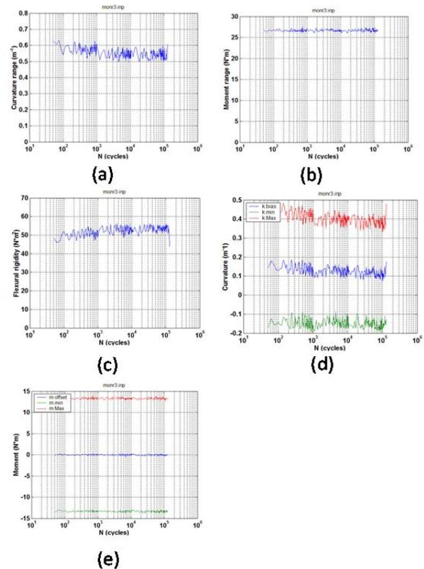
Fig. 2. Variations of (a) curvature range, (b) applied moment range, (c) flexural rigidity, (d) maximum and minimum values of curvature, and (e) maximum and minimum values of moment as a function of number of cycles for D13/R3 (606B3E);  $N_f = 1.29 \times 10^5$  cycles under  $\pm 13.72 \text{ N}\cdot\text{m}$  5 Hz.
