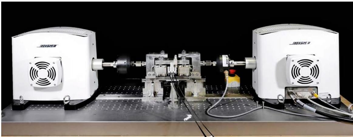
Fig. 1 Cyclic integrated reversible-bending fatigue tester, where the SNF is loaded in the central U-bent fixture
