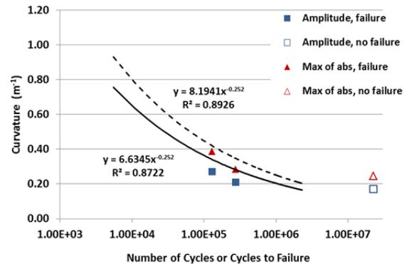
Fig. 4. Maxima of absolute (abs) curvature extremes and curvature amplitudes as a function of number of cycles. Solid markers represent tests with specimen failures; open markers indicate tests without failures. The power function was obtained from curve fitting based on the HBR data set [5]; solid line corresponds to amplitudes, and dash line corresponds to maxima of absolute.
