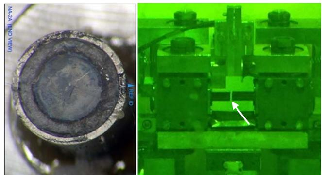
Fig. 10. Failure cross-section and fracture location of NA2 (651C5),  $N_f = 2.2 \times 10^4$  cycles under  $\pm 10.16$  N·m.
