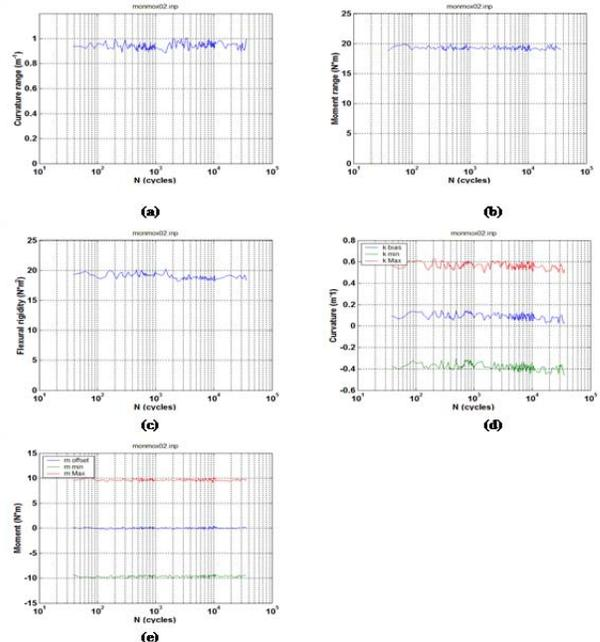
Fig. 14. Variations of (a) curvature range, (b) applied moment range, (c) flexural rigidity, (d) maximum and minimum values of curvature, and (e) maximum and minimum values of moment as a function of number of cycles for MOX2 (MOX-A-12).
