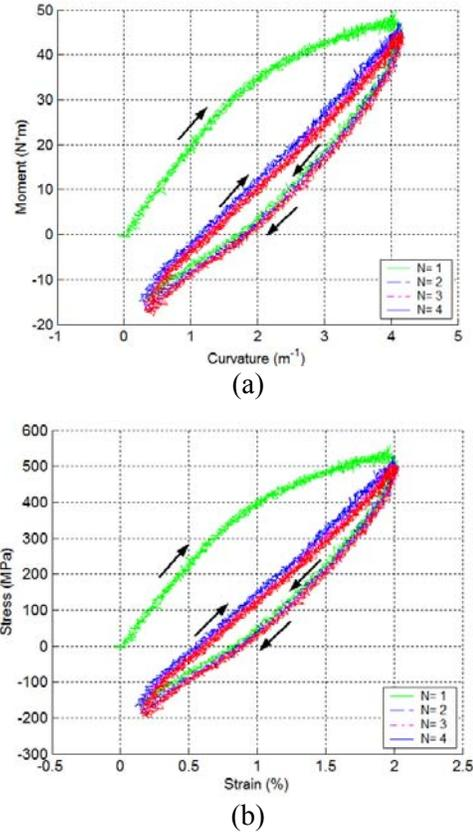
Fig. 6. (a) Moment-curvature curves and (b) equivalent stress-strain curves based on the first four loading cycles for specimen NA3 (651D3).
