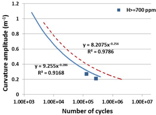
Fig.5. Curvature amplitudes as a function of number of cycles or  $\kappa$ -N curve for HBR used fuel with various levels of hydrogen content. The power function was obtained from curve fitting based on the HBR data set; the solid line corresponds to  $H \geq 700$ ppm, and the dashed line corresponds to  $H < 700$ ppm [5].
