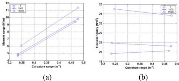
Fig. 12. (a) Moment-curvature relation and (b) moment-flexural-rigidity relation at various numbers of cycles for MOX (MOX-A-12). Measurements were made with 0.8 and 1.6 mm relative displacements;  $N_f = 3.7 \times 10^4$  cycles under  $\pm 10.16 \text{ N}\cdot\text{m}$ , 5 Hz.
