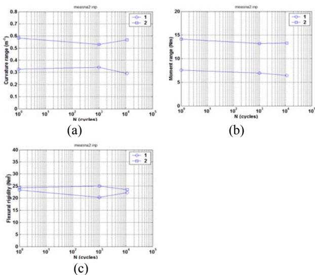
Fig. 8. Variations of (a) curvature range, (b) moment range, and (c) flexural rigidity as a function of number of cycles for NA2 (651C5). Measurements were made with 1.0 and 2.0 mm relative displacements;  $N_f = 2.2 \times 10^4$  cycles under  $\pm 10.16$  N·m, 5 Hz.
