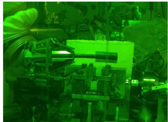
Fig. 7 Image of specimen NA3 (651D3) after testing; the rod sustained four cycles of loading to 24.00-mm relative displacement; the maximum moment with a level of 47 N·m was reached during the initial loading cycle.
