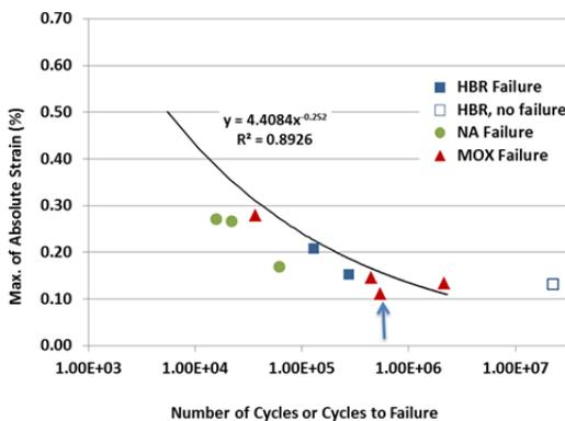
Fig. 16. Maxima of absolute strain extremes as a function of number of cycles; results are based on CIRFT testing at 5 Hz. The power function was obtained from curve fitting
