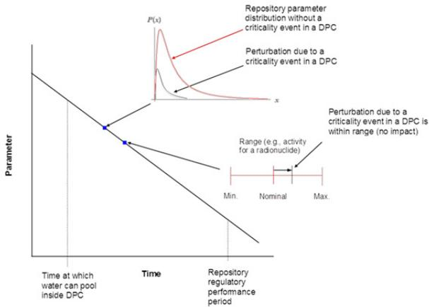
Fig. 2. Illustration of consideration of criticality consequences on PA parameters.
