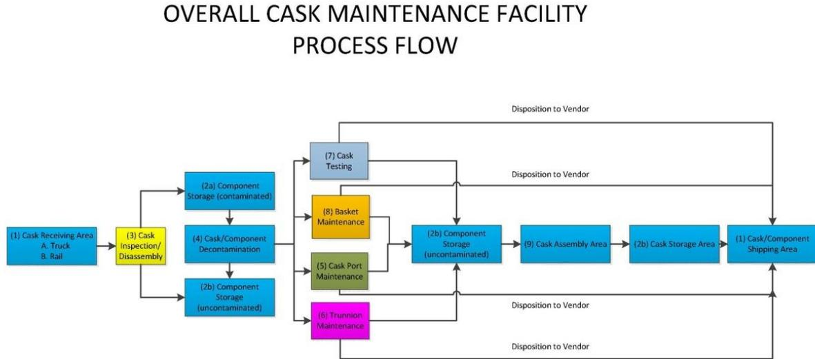
Fig. 6. Cask Maintenance Process Flow Flowchart (conceptual view)
