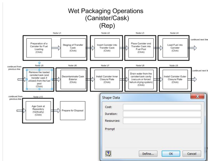
Fig. 2. Example node Visio property values with links to cell values in Excel (conceptual view)
