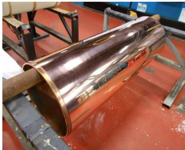
Fig. 1. Free-standing copper shell produced by electroforming at BEP Surface Technologies Ltd. Dimensions: 1 m diameter, 2.5 m long and 16 mm wall thickness.
