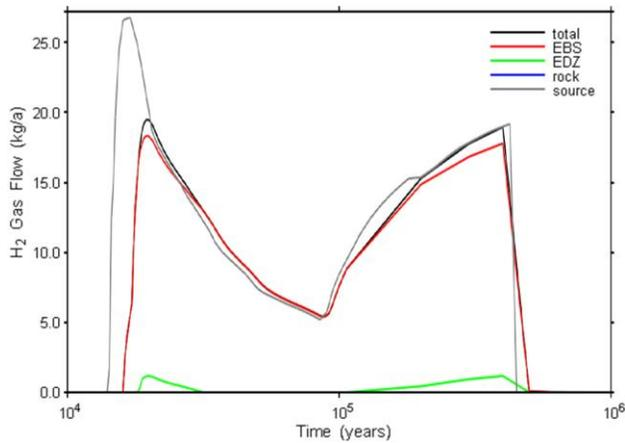
Fig. 8. The Repository-Scale Model – Gas Flow Out of the Top of the Model
