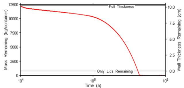
Fig. 3. The Room-Scale Model – Steel Consumption
